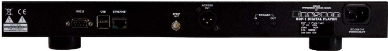
of trigger connectors and to the very right is the IEC a.c. power connector.
